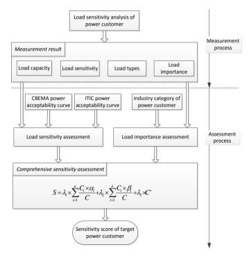
Fig. 1. The steps of customer sensitivity assessment under voltage sag disturbance
