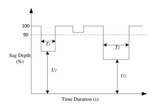
Fig. 2. The two-dimensional region to describe the intensity of sag disturbance
