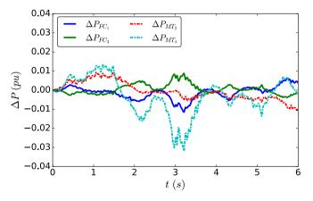
Fig. 9. Power deviations of FCs and MTs.
