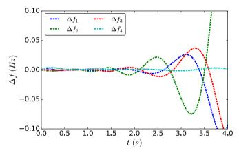
Fig.2. Frequency deviations without control (no disturbance input).
