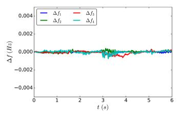
Fig.8. Frequency oscillations with robust  $H_{\infty}$  controller (with disturbance input).
