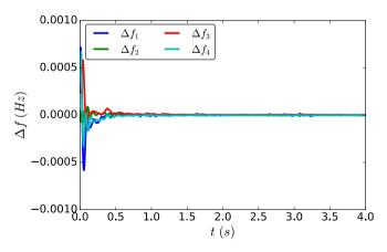
Fig.3. Frequency deviations under robust controller (no disturbance input).
