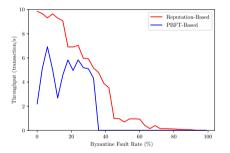
**Figure 10:** Throughput comparison between delegated consensus-based blockchain and PBFT-based blockchain as the Byzantine fault rate increases.
