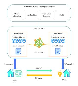
**Figure 5:** Architecture of P2P energy trading system based on blockchain and reputation.
