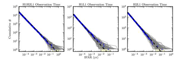
FIG. 1: The cumulative distribution of events above a threshold IFAR, for in-time coincident events, shown as blue triangles, from all coincidence categories for the observation times H1H2L1, H1L1, and H2L1 respectively. The expected background (by definition) is shown as a dashed black line. The 100 experimental trials that make up our background are also plotted individually as the solid grey lines. The shaded region denotes the  $N^{1/2}$  errors.
