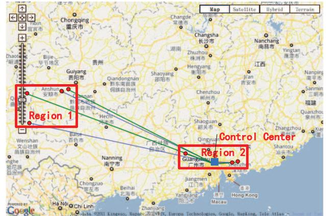
Fig. 8 WAMC system of the China Southern Power Grid.
