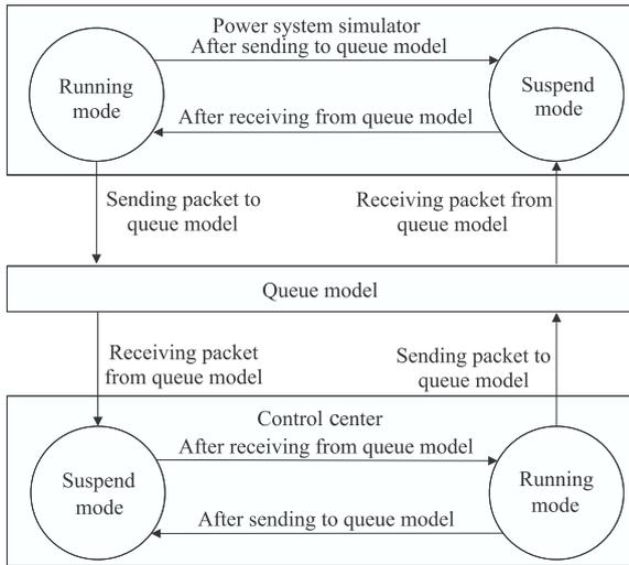
Fig. 2 System state diagram.
