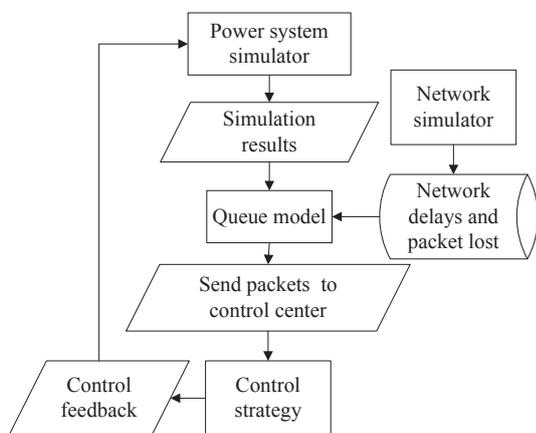
Fig. 1 The integrated cyber-physical simulation framework.
