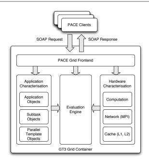
**FIGURE 3.** Key PACE components. Clients connect to a PACE *performance service* which runs inside an OGSA/OGSI container. This in turn compiles, caches and evaluates model objects using the PACE back-end tools.
