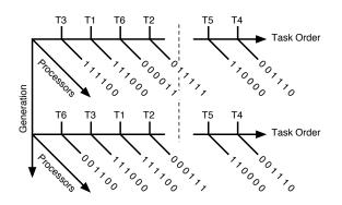
**FIGURE 5.** The crossover operator which merges the tail of one schedule with the head another. Where tasks are duplicated, the crossover process is reversed.
