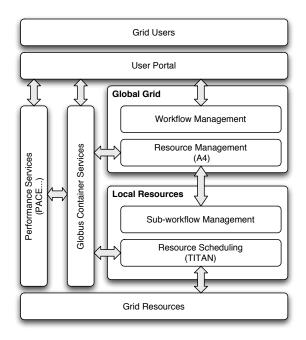
**FIGURE 2.** Key components in the TITAN architecture. Workflow descriptions are submitted to a broker, which locates a suitable resource set and passes the sub-workflow scripts to a local scheduler.
