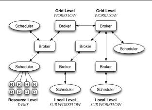
**FIGURE 1.** The multi-tiered workflow management architecture. Grid level is used to describe inter-domain resource balancing. Local level is used to describe the mapping of tasks to resources.
